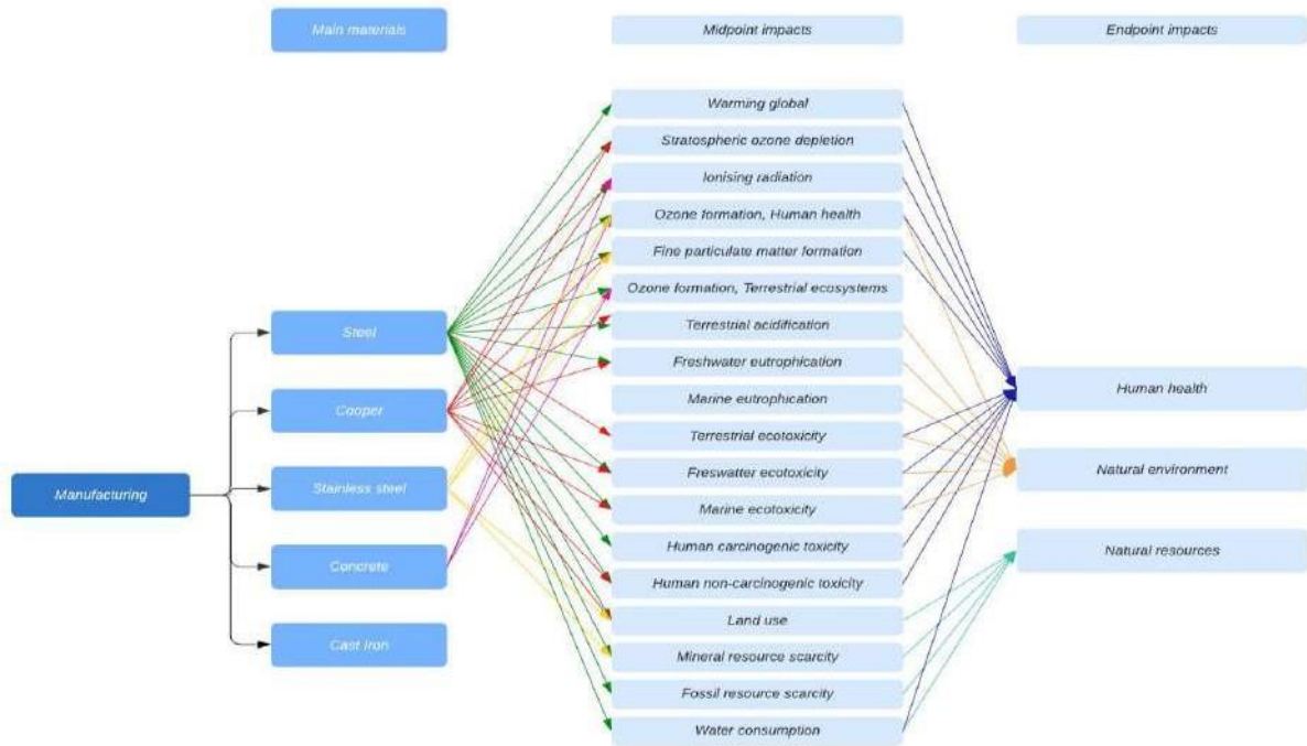
Fig. 2. Relationship between major metallic and non-metallic materials and the environmental impacts identified by the 18 midpoint and endpoint impact categories.
