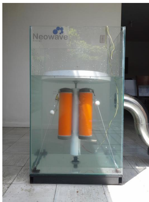
Fig. 2. Small scale functional model, and water level change mechanism after concluding the home-made tests.
